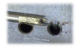
**Note**: Marks on right side of the hole where caused by breaking off the taps manually. Not by the drilling process.
